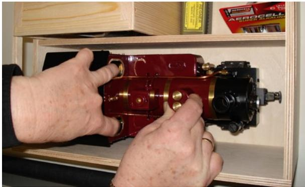
The locomotive can be taken out of the case by lifting it at the steam dome and two fingers trough the front window openings.
